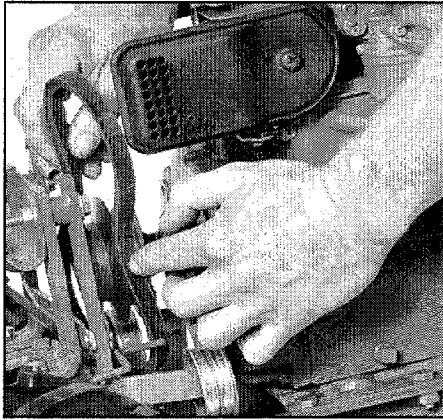
Figure 5-17: Install forward drive belt over rear of engine forward pulley and bring lower half of belt down and in front of transmission pulley.
